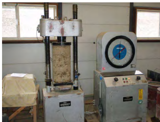
Photo-13 Strength Test of CSG Specimens (In Laboratory)
