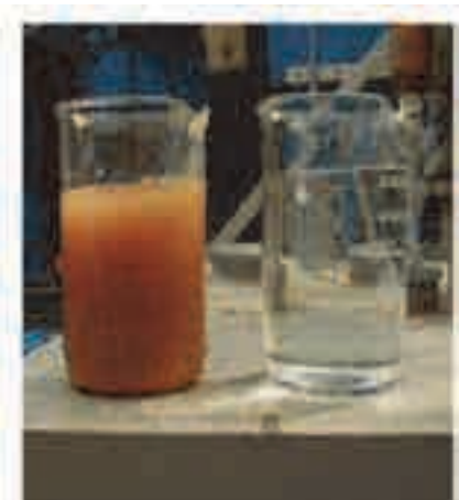
Raw water and treated water
