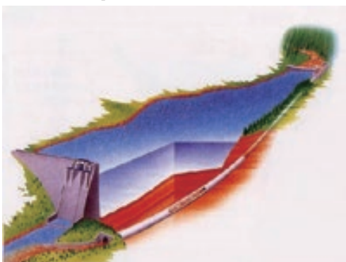
Figure-3 Sediment bypass tunnel (SBT)
