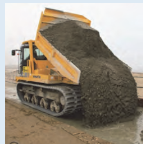
Transportation Dump Trucks (10t class Crawler type)
