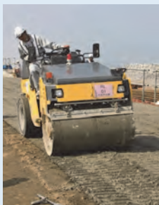
Compacting Vibrating Roller (4t class combined type)
