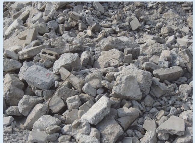
Stock Yard of Concrete Wreckage (Raw Materials of CSG)
