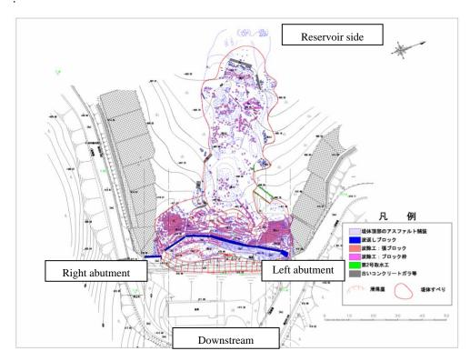
Figure 3. Damage of structure and slides of auxiliary dam
