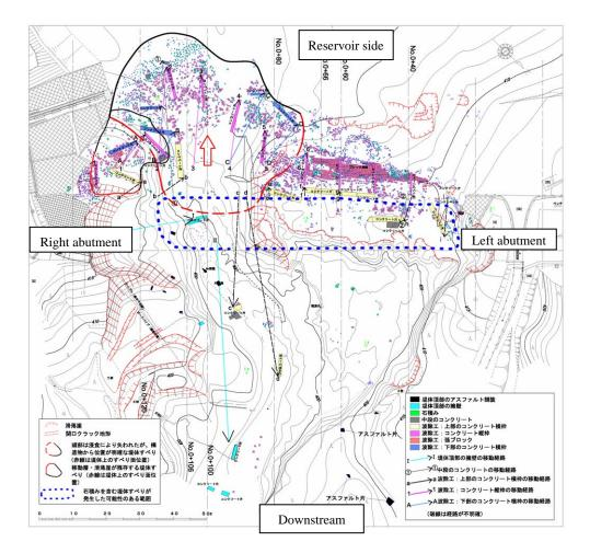
Figure 1. Mapping of structural elements after failure
