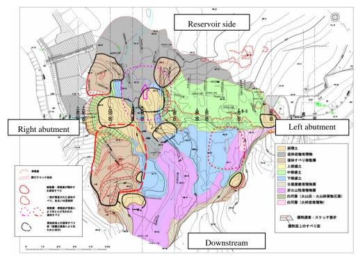
Figure 2. Possible slides estimated from geologic and topographic mapping Notes: Encircled lines indicate the slide block.
