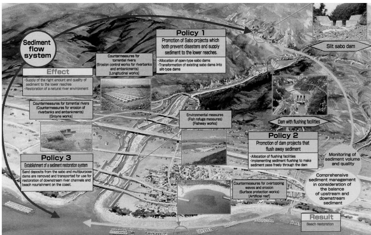
Figure 2 Conceptual diagram of Kurobe River comprehensive sediment management
