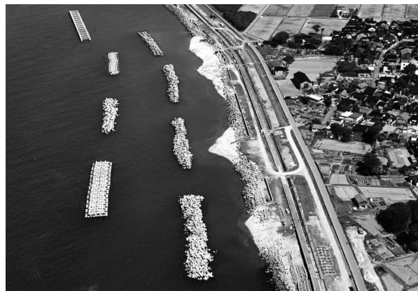
Photo 3 Establishment of offshore breakwaters (Yoshiwara District in Nyuzen Town)
