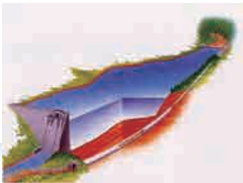
Figure-3 Sediment bypass tunnel (SBT)
